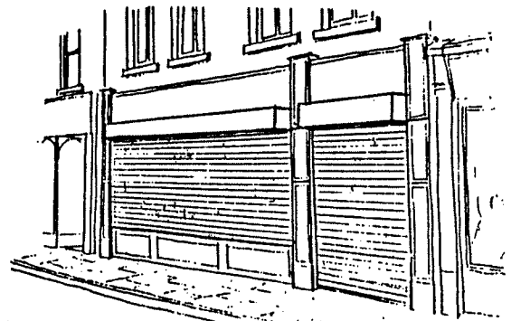
Both external roller shutters and external shutter boxes are NOT ACCEPTABLE . Planning Permission and Listed Building Consent will be required.
