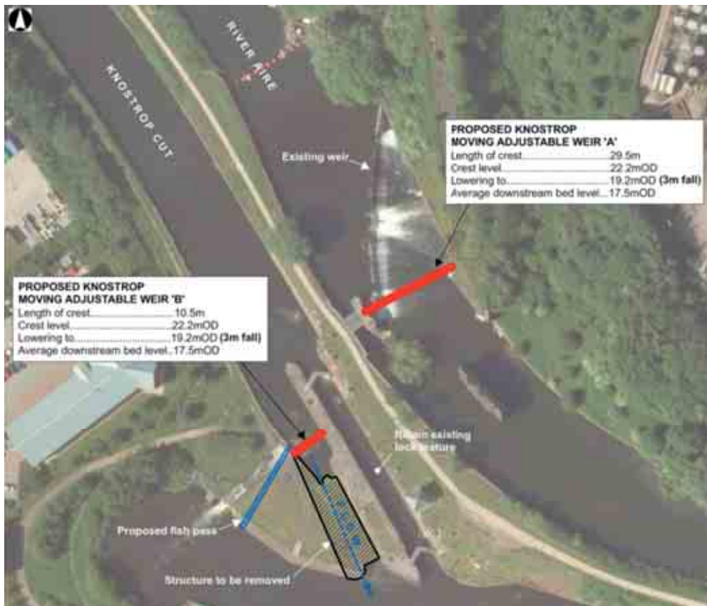
Leeds Flood Alleviation Scheme: Proposal for Movable Weir – concepts courtesy of Arup
